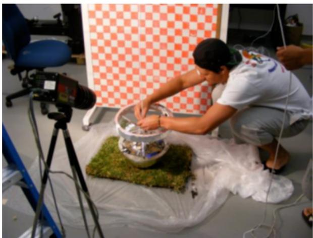
Figure 3. Prepare test for landing on grasses
