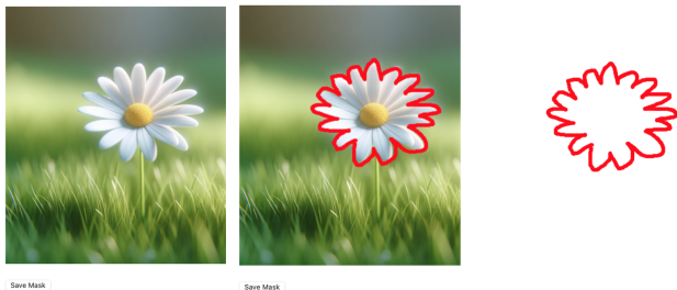
Figure 13: Screenshot of the GUI generated by Method 5. This figure includes the original image (left), the user-annotated image (middle), their respective save buttons below each, and the saved mask after pressing the save button (right).
