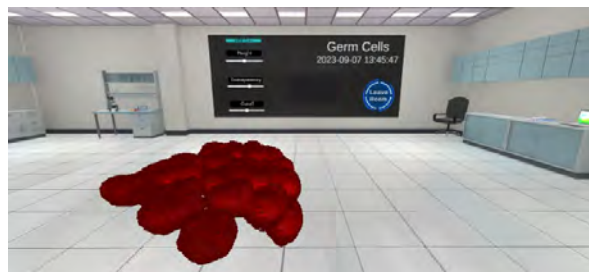
Figure 2. 3D cell model in networked visualization application. Cell images are loaded into the lab environment and compiled into a 3D model. The user interface (UI) located on the board displays all relevant cell information as well as the slider interface that is able to transform the 3D cell model. The lab scene provides a comfortable environment for working with the model as well as provides a professional feeling to the application.
