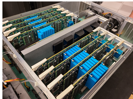
Figure 1: An internal view of the Lucata Pathfinder chassis.
