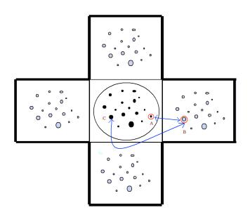
(2.3) Illustration of a "wrapped" world as is pertains to the code. The distance between particle A and B represents the "ghost" distance. Particle B does not exist because we are dealing with a "wrapped" world. Therefore, the "real" distance is between particle A and C.
