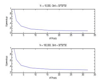
(4.2) Above are the Speedups of the Wall-times of GalaxSeeHPC as a function of the # of processors. The speedup value is calculated by divided the wall-time of P processors by the wall time for one processor.
