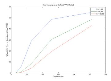
(5.2) The above graph is the Percentage of total time spent in PrepPPPM as a function of the Grid Resolution. The time in computing the Fourier Transform increases as the mesh size increases.
