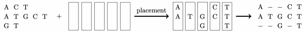
Figure 4: CAF aligns sequences by assigning the elements in each sequence a column and inserting gaps into any column spaces with no elements [24].
